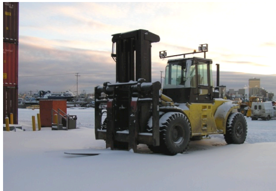
31-ton short-mast forklift
